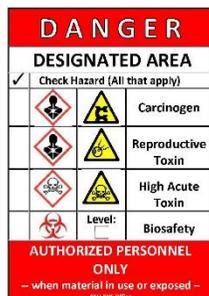
The picture above shows the BSU *Designated Area* sign. The appropriate hazard characteristic(s) of the chemical(s) are to be checked and the adhesive label applied as necessary to demarcate the allowable area in which the chemical may be used or exposure may occur. The label may also be placed on cardstock or a tag for display. **Note:** The same sign may also be used to designate areas subject to Biosafety Level controls for infectious materials.
