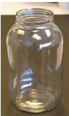
Clear Standard Wide Mouth Bottles with PTFE-faced PE-lined Caps Good for storing dry materials and specimens
