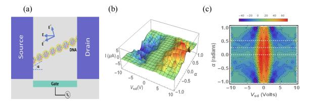
Figure: (a) Tilted DNA channel between source and drain contacts, (b) Current as a function of a source-drain voltage and tilted angle, and (c) differential conductance as a source-drain voltage and tilted angle.
