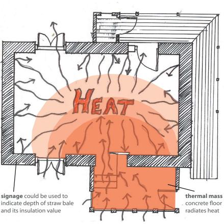
Thermal efficiency of the LandLab building relies on the thickness of the walls as well as the sunroom space. The thick straw bale construction has a high insulation value that traps heat within the building during the day. This heat is maintained throughout the night. The concrete slab in the sunroom also serves as a thermal mass that can be released during the night into the main living and working space.
