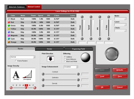
14) For each color you used in your document, the **Mode** needs to be set to **Vect** (typical) or **Rast** (less often used) and the **Power**, **Speed** and **PPI** values need to be set according to the sample cut card for the material you are cutting.
