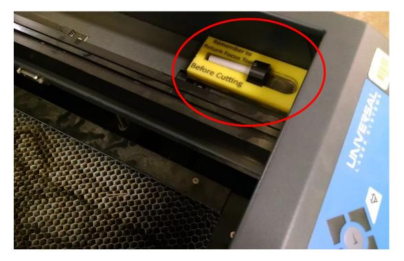
23) Place the focus tool on top of the material, near the laser focus carriage. Raise or lower the bed using the UP and DOWN buttons on the machine so that the lower corner on the flat side of the focus tool rests against the lower front corner of the focus carriage. See below.
