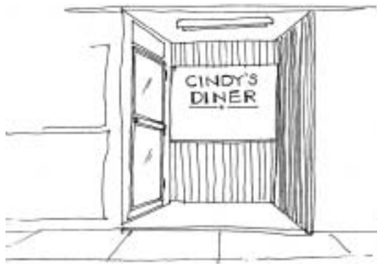
Poorly altered entryway: door relocation, modern door with no windows.
